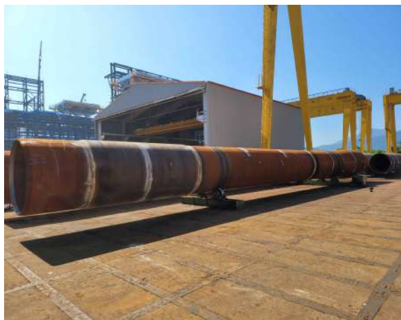
The production of thick-walled pipes has been completed (Storage yard for thick-walled pipe products)
