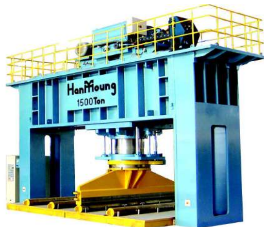
RT Press (For Bow and Stern Work on Ships)
