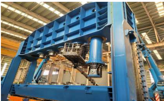
On-site Assembly of Press Brake
