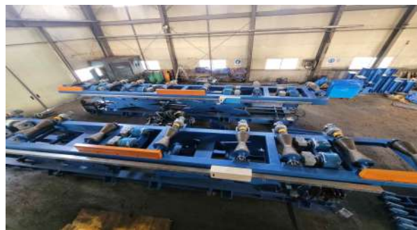
JCO Method Pipe Feeding System Fabrication Process
