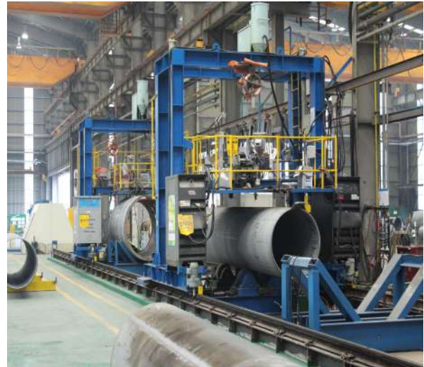
Delivery to Guman Heavy Industries (Pipe Manufacturing Internal and External Welding Machine)
