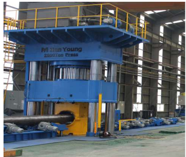
Delivery of 2,500-ton Press to Gunsan Shipbuilding & Marine Technology Business Cooperative (Pipe Manufacturing Production Equipment)
